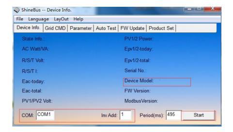
Then in "Product Set" page, fill in AxB1DxTxPFU1MxSx, only change B0 to B1 to enable export limitation function, keep others same as the model value you record, for example, if record model value is A0B0D0T0PFU1M8SA, then fill in A0B1D0T0PFU1M8SA, and click Set to save the setting.
