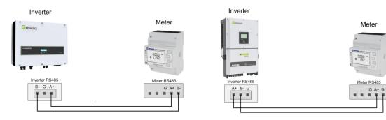
3-15KTL3-S inverter and meter connection
