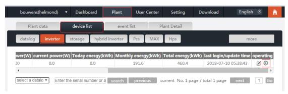
Click "advance set", select the register, and fill in 202 and value 1 as below picture, then fill in the password and click "save", to enable this setting.
